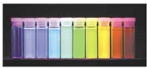
Figure 15: Ten distinguishable emission colours of ZnS-capped CdSe quantum dots excited with a near-UV lamp: from left to right (blue to red), the emission maxima are located at 443, 473, 481, 500, 518, 543, 565, 587, 610, and 655 nm
