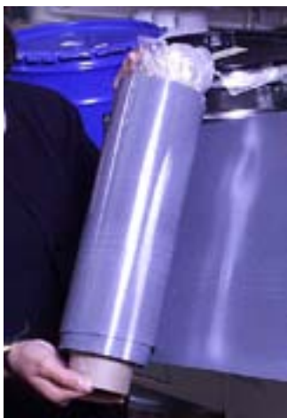
Figure 5: Rolled up Gyricon e-paper
