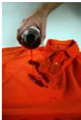
Figure 7: Liquid staining on a Nano-Tex® fabric
