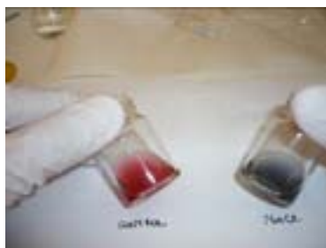
Figure 11: Colour change as salt is added to the gold colloid
