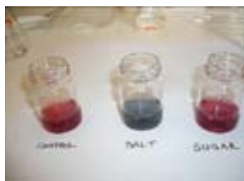
Figure 13: Effect of adding a solution of sugar to the gold colloid (vial on the far right). The middle shows the vial to which salt solution was added to the gold colloid, and on the left is a control (pure gold colloid).
