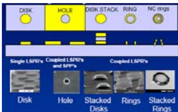
Figure 7: Summary of the various nanostructures that can be formed as regular arrays on surfaces
