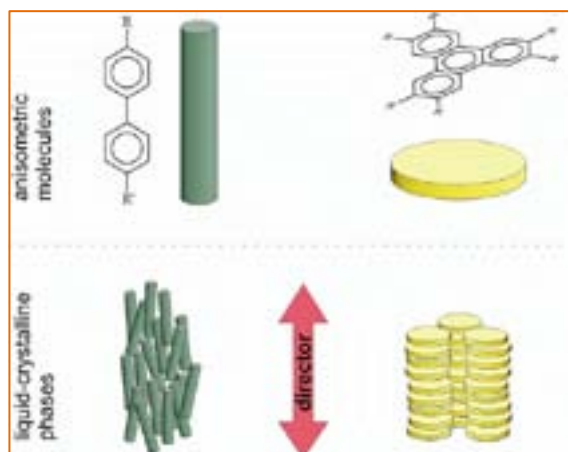
Figure 2: Examples of the self-organisation of anisometric (i.e. with asymmetrical parts) molecules in liquid-crystalline phases: (left) rod-like molecules form a nematic liquid, in which the longitudinal axes of the molecules are aligned parallel to a common preferred direction (director); (right) disc-like (discotic) molecules arranged into molecule-stacks (columns), in which the longitudinal axes are also aligned parallel to the director. As a result of their orientational order, liquid crystals exhibit anisotropic physical properties, just like crystals.
