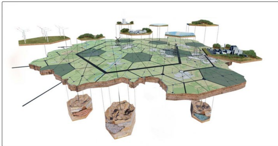
Figure 19. Design of a spatial scenario in which the use of salt caverns for storage of sustainable energy can provide an (inter)national energy hub in the Netherlands. 19
