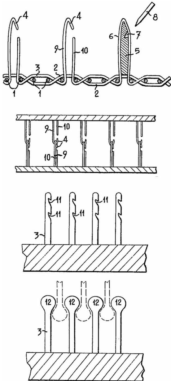
**Fig. 4** Drawings from the 1951 patent application for a 'Velvet type fabric and method of producing same' showing different possibilities for reversible attachment systems. Source: <http://v3.espacenet.com/origdoc?DB=EPODOC&IDX=CH295638&F=0&QP=CH295638>
