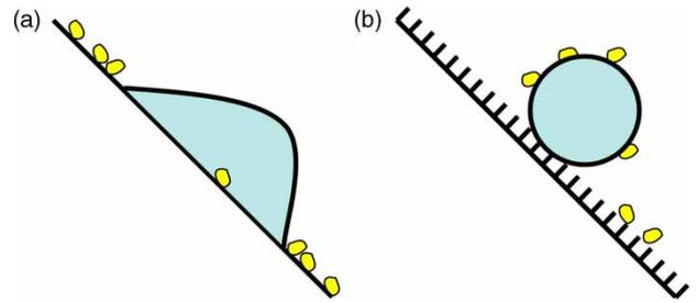
**Fig. 5** Schematic diagram: (a) on a conventional flat surface, the liquid droplet slides over the dirt and only redistributes the particles; (b) on a self-cleaning surface, the dirt particles have only small contact area with the surface, and the large contact angle of the liquid droplet causes the droplet to roll over the surface, with the dirt particles adhering to the droplet
