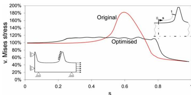
**Fig. 3** Biomimetically optimized straw bale screw: The diagram shows the von Mises stress before and after optimization of the radius in the thread. The stress is reduced by more than one-third compared to a conventional radius for the case of load shown in the inset. Diagram and inset reproduced from reference [13] with permission ©Springer 2006
