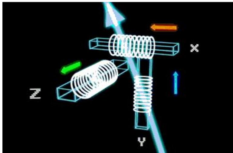
Figure 14: 3D-Measuring with three Fluxgate magnetometers [13]
