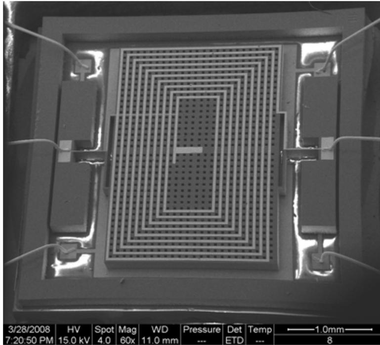
Figure 15: Image of planar interwining magnetic coils wrapped around the magnetic core material
