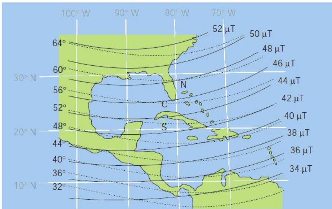
Figure 7: Equivalent circles of the fields strength and the inclination at the Gulf of Mexico [9]
