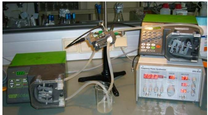
Fig 11: Experimental set-up of ultrasonic separation
