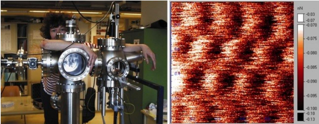
Figure 1. *Left: An ultrahigh vacuum atomic force microscope combined with a scanning tunnelling microscope (UHV AFM/STM). Right: Atomic force microscopy image of the surface of a highly oriented pyrolytic graphite (HOPG) crystal, image area  $1 \times 1 \text{ nm}^2$ .*
